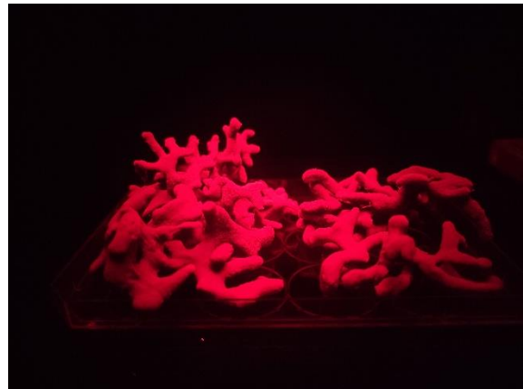
Figure 9 - Actinic light over a sample of Codium during photosynthetic activity measurement using Walz Imaging PAM
