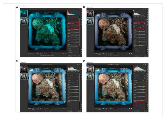
FIGURE 3 | Demonstrating the irrelevance of the Infrared Cut Filter. (A) Raw image taken with ICF on the camera port. (B) The same image from A after white balance (WB) correction in post processing using adobe camera raw (Adobe, United States). (C) Raw image taken without ICF shows the correct colors without the need of WB correction. (D) The same image from C after automatic editing tool using adobe camera raw (Adobe, United States). Red box indicates the command setting.
