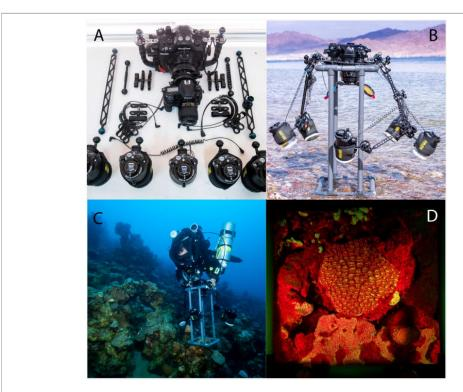
FIGURE 1 | (A) Complete gear set of Nauticam housing, Nikon D850 camera with 35 mm lens, strobes and arms before assembly. (B) The complete set assembled on the quadrat before diving. (C) A diver equipped with closed circuit rebreather and the speed-FloriS at 45 m in Bermuda. (D) An example of stony coral's image taken in Bermuda at daytime at 45 m with the fluorescence excitation strobe without subtraction.
