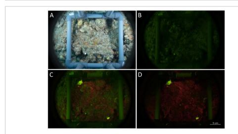
FIGURE 5 | Images set taken with the speed-FlorIS. (A) Reflectance image taken under white illumination, (B) ambient image (blue strobes off), (C) fluorescence image (blue strobes on), and (D) fluorescence image after subtracting image (B) from image (C) using Fiji software (Schindelin et al., 2012).
